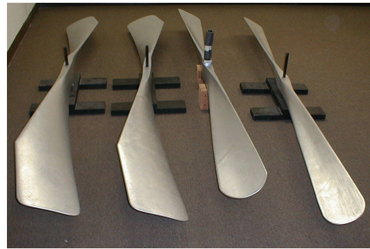
Figure 1. Photograph of Wright Brothers propeller reproductions between 1911 (left) and 1903 (right). Propeller lengths are 8 ft. 6 inches.
